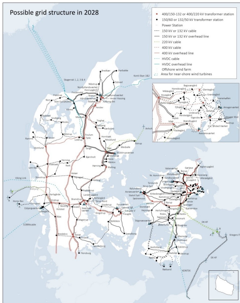
Figure 38. Possible electricity transmission grid structure by 2027 drafted by the Danish TSO, Energinet (Energinet, 2018)
